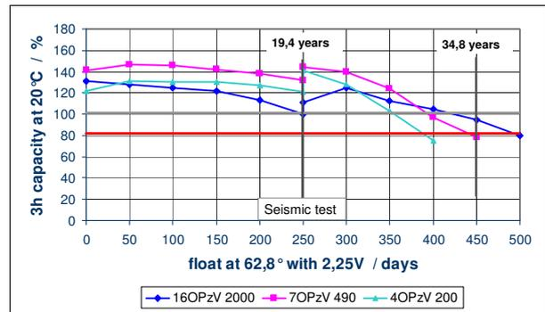
Fig. 9 OPzV 3h capacities within 450 days at 62,8°C
