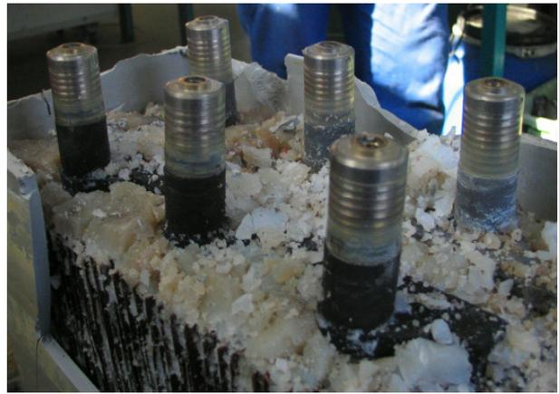
Fig. 13 OPzV 2000 opened after 450days at 62,8°C
