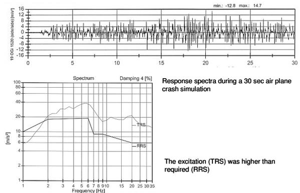
Fig. 3 Response spectra during the airplane crash simulation.
