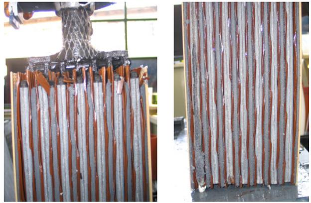
Fig.8 OPzS plates set after 550 days at 62,8°C
