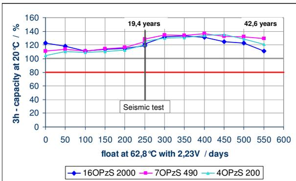
Fig. 5 OPzS 3h-capacities within 550 days at 62,8°C
