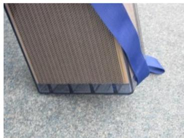
Tilt the cells slightly and position the blue strap centralized on the cell bottom.
