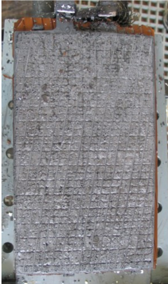
Negative plate 2.8% \text{PbSO}_4
